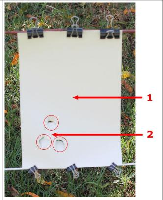
If the distance between arrow 1 and arrow 2 is very small, then just adjust the sticker on the Hand Controller to be on arrow 2. The spares bag has additional stickers.
